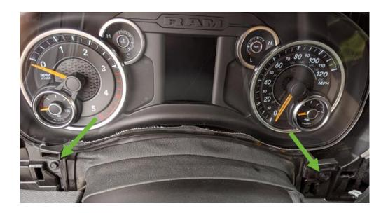
5. Remove four 7mm screws that hold the instrument cluster in place and remove the cluster.
