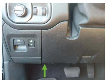
2. Disconnect the two connectors from the security gateway module and insert the connectors into the STE pass through connector. Ensure that both connectors are fully seated into the pass the pass through by pressing on the backs of the connectors.
