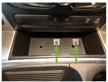
3. Remove one 8mm bolt from the mid compartment.
