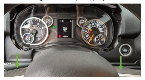
4. Remove two 7mm bolts that hold the steering wheel boot bracket.
