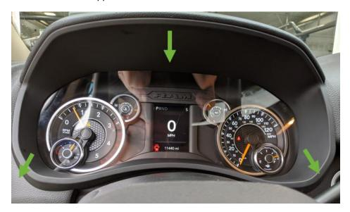
3. Remove the left and right lower bezel trim pieces by pulling towards the rear of the vehicle.
