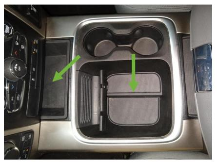
2. Remove two phillips screws from the front compartment.
